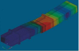
Based on that, a finite element model was carried out to simulate the experiment. The main goal of this simulation was to get a better understanding of the coupling system mechanical behavior. It was calculated with two different finite elements programs; Tochnog and Abaqus. Moreover the concrete was calculated with two different material models as well; the material constitutive subroutine developed by Züblin (UMAT) and the concrete damaged plasticity theory provided for Abaqus.
