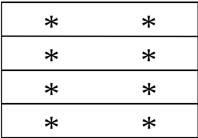
Figure 7-3 Integration Points through the Thickness of Continuum Composite Elements
