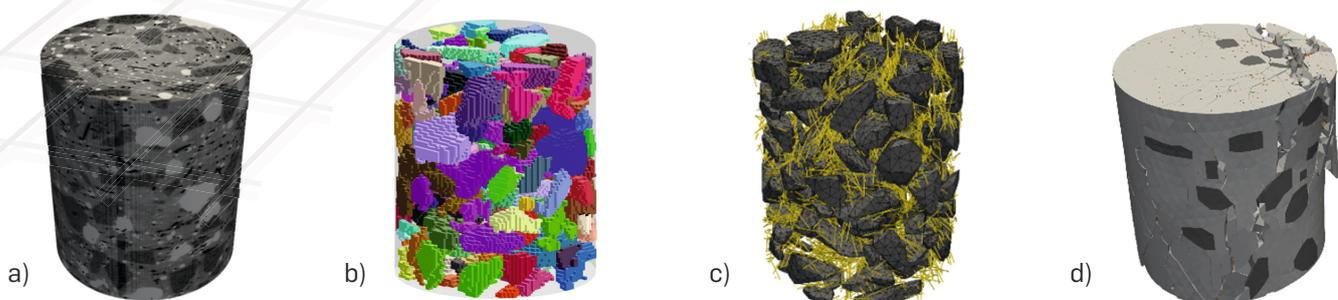
Fig.: Generation of the computational model from a CT image: (a) Original CT image of an actual sample showing four phases: fibers (black), aggregates (dark gray), mortar matrix (gray), and air voids (light gray). (b) Identification of individual aggregates. (c) Isolated aggregates (dark gray) and fibers (yellow). (d) Numerically obtained fracture pattern.
